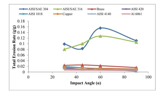
Figure 8. Total erosion rate against impact angle
