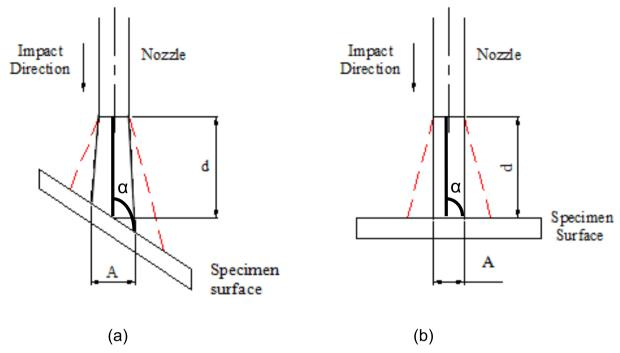
**Figure 5.** Impact geometry, (a)  $\alpha \le 45^{\circ}$ , (b) Near or at  $90^{\circ}$
