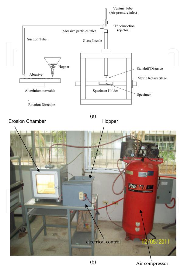
Figure 2. (a) Schematic Diagram of erosion rig developed, (b) Experimental setup [8]
