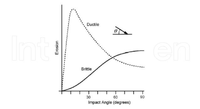
Figure 9. Erosive wear rates for brittle and ductile materials [4].
