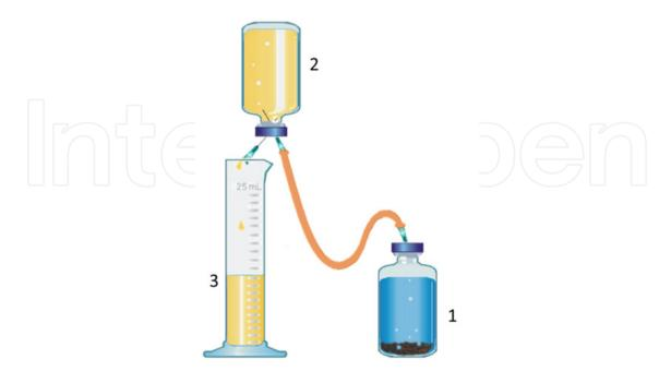
**Figure 2.** Schematic representation of methane measuring displacement of a solution of 3% NaOH. 1) serological bottle, 2) serological bottle with 3%NaOH 3) test tube to measure the displaced NaOH
