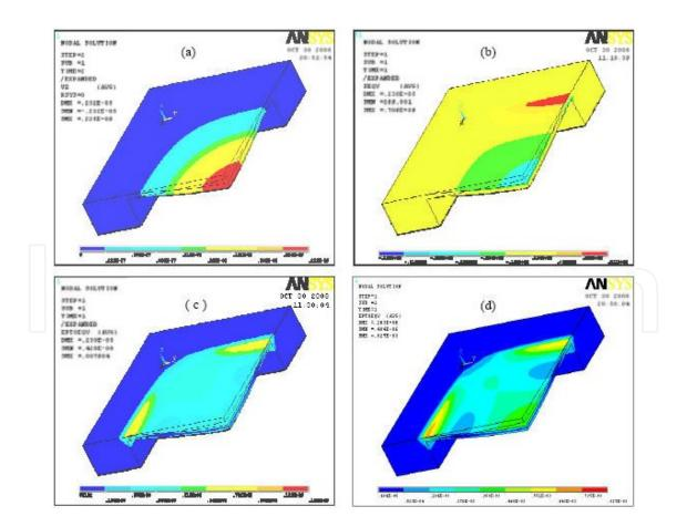
Figure 10. The simulation result from ANSYS (a) displacement; (b) stress in x direction; (c) stress total; (d) strain.
