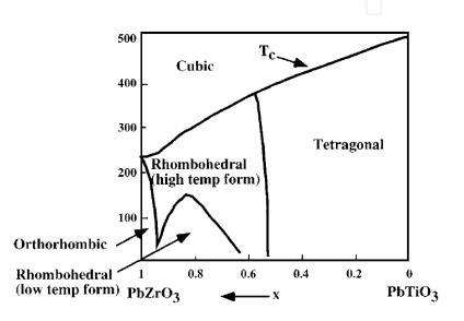
**Figure 2.** Phase diagram for the PbZrO3-PbTiO3 system (from Ref. [9]). The nearly vertical phase boundary between the rhombohedral and tetragonal phases is called the morphotropic phase boundary.
