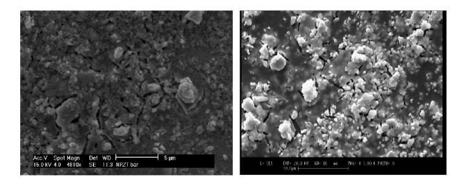
Figure 7. SEM morphology of PZT composite films. Mass ratio of powder to solution: (a) 1/4, (b) 1/2
