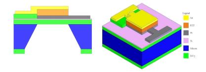
Figure 8. Structure and Cross section of the multilayer PZT diaphragm.
