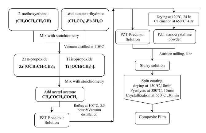
Figure 3. Flowchart of preparation PZT composite layer
