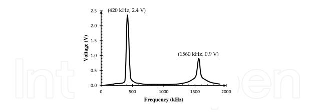
Figure 15. Voltage response in PZT-layer at centre point of the diaphragm
