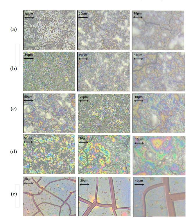
Figure 6. Optical microscopic pictures. Mass ratio of powder to sol is (a)  $\frac{1}{1}$ , (b)  $\frac{3}{4}$ , (c)  $\frac{1}{2}$ , (d)  $\frac{1}{4}$  (e) without powder
