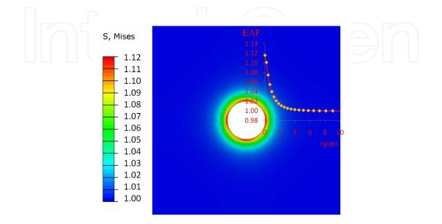
Figure 10. von Mises stress contour and 'EAF vs. distance' curve [39].
