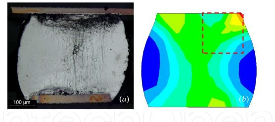
**Figure 11.** *a*) Plastic deformation of the solder interconnection after 1000 thermal cycles, (*b*) FEM-calculated inelastic strain energy density distribution, dashed rectangle shows the domain of the microstructural simulation [39].
