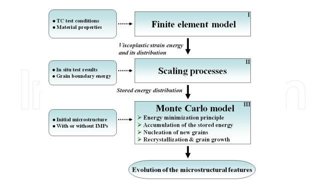
Figure 5. Flow chart for the simulation of microstructural changes in solder interconnections [39].
