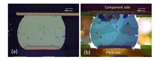
Figure 3. Micrographs of the solder interconnection after 6000 thermal cycles; (a) optical bright field image, (b) cross-polarized light image.
