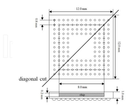
Figure 6. Schematic show of the BGA component under study [39].
