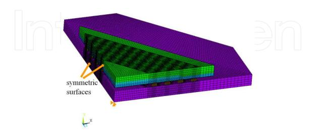
Figure 7. Finite element model for the thermomechanical calculation [39].
