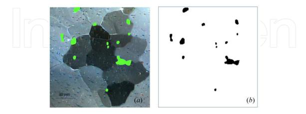
**Figure 13.** *a*) Micrograph shows IMP-affected recrystallization, (*b*) initial microstructure for the Monte Carlo simulation [39].
