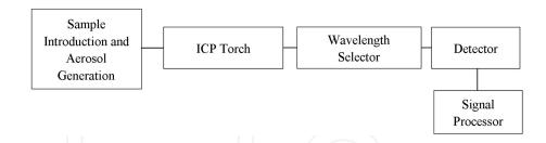
Figure 2. Block Diagram of ICP-OES.
