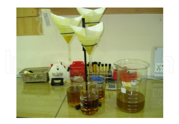
Figure 7. Biodiesel Filtration
