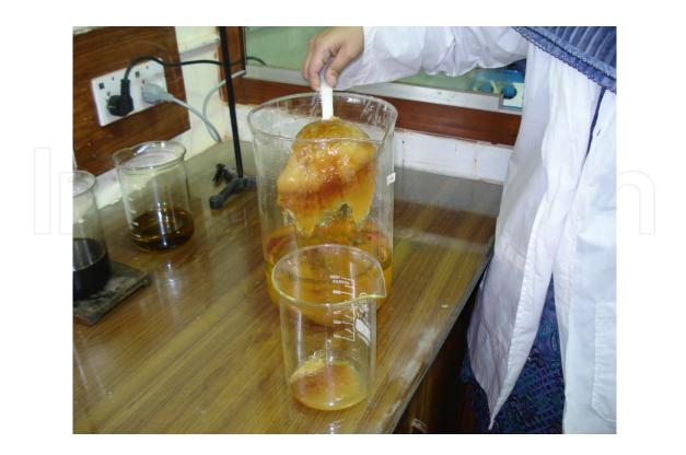
Figure 6. Separation of glycerin from Biodiesel
