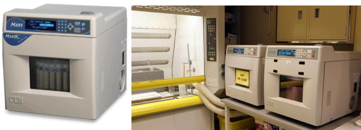
**Figure 1.** Typical equipment (MARS), used for MW hydro/solvothermal processing.
