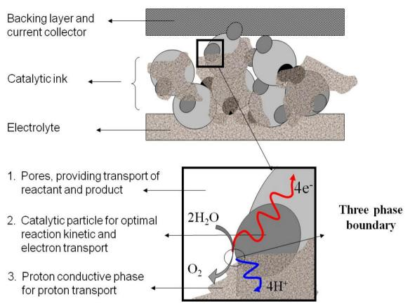
Figure 1. Schematic overview of the three phase boundary
