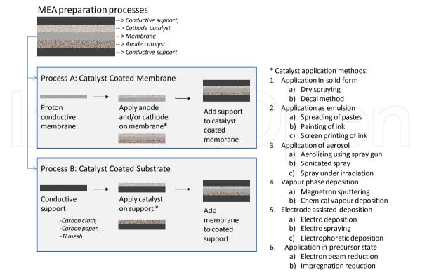
Figure 2. Schematic of catalyst-coated GDL (CCG) and catalyst-coated membrane (CCM) structures.
