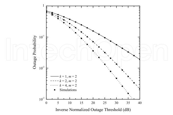
**Figure 2.** Outage Probability of SISO receivers employing intensity modulation and direct detection and operating over G - G channels, for different values of parameters *k* and *m*, as a function of the Inverse Normalized Outage Threshold,  $\overline{\mu}/\mu_{th}$ .
