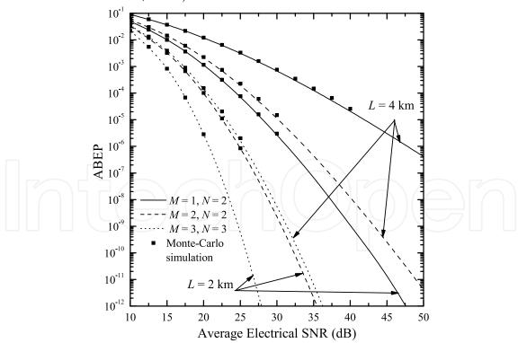
**Figure 7.** ABEP of MIMO FSO systems employing EGC and operating over i.i.d G – G fading channels as a function of the average electrical SNR, ( $\lambda = 1550$ nm,  $C_n^2 = 1.7 \times 10^{-14}$ m<sup>-2/3</sup> and  $D/L \rightarrow 0$ )
