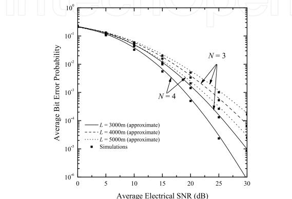
**Figure 4**. ABEP of triple and quadruple branch SIMO FSO links operating over exponentially correlated G - G atmospheric turbulent channels and employing optimal combining, versus average electrical SNR  $\mu$  for  $\rho = 0.175$  and different link distances.
