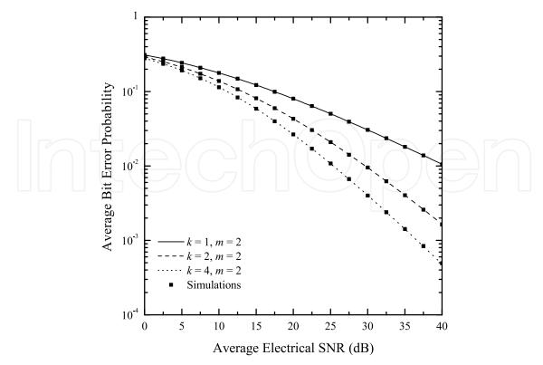
**Figure 1.** Average Bit Error Probability of SISO OOK receivers employing intensity modulation and direct detection and operating over G - G channels, for different values of parameters *k* and *m*, as a function of the Average Electrical SNR,  $\overline{\mu}$ .
