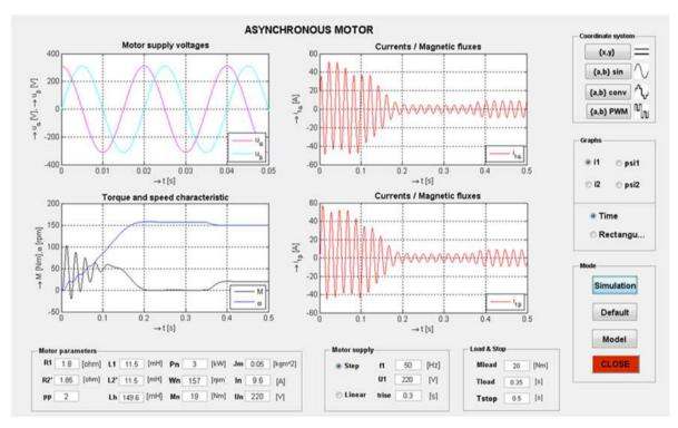
Figure 12. GUI screen of the AC drive with induction machine
