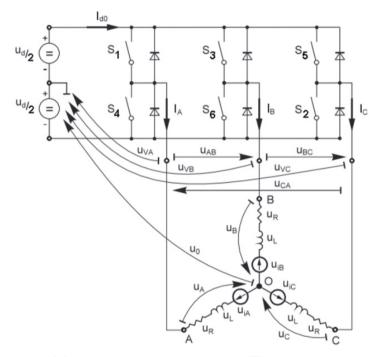
Figure 14. BLDC motor model
