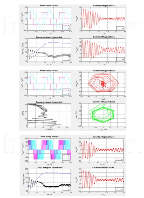
Figure 13. Examples of diplaying various graphs in the GUI for asynchronous motor
