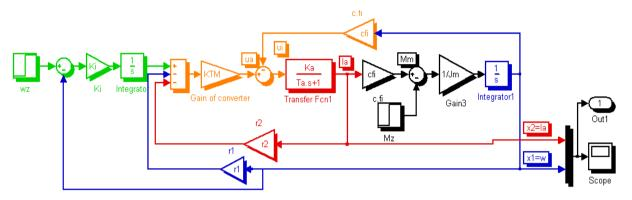
Figure 23. Simulink model of the state-space control of DC drive
