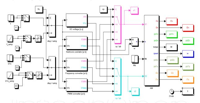
Figure 11. Arrangement of asynchronous motor subsystems in the Simulink GUI model
