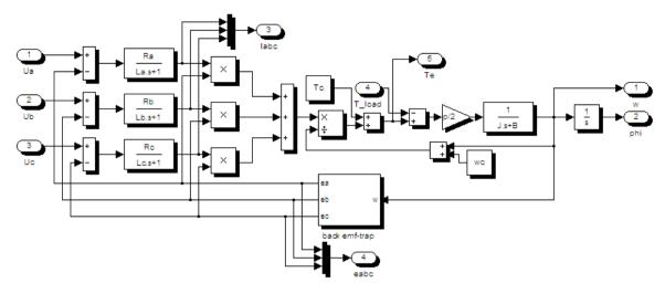
Figure 16. Detailed overview of the BLDC motor block
