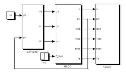
Figure 15. Simulink model of the BLDC motor
