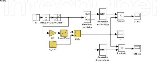
Figure 7. The model of converter realizing the frequency starting under consideration of the law of constant stator flux (U/f = const.)
