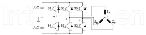
Figure 18. Modelled three-phase converter
