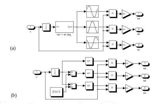
Figure 17. Trapezoidal (a) and simusoidal (b) model of the back-EMF
