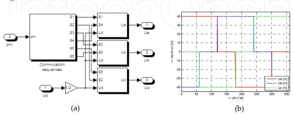
Figure 19. Detailed overview of the three-phase converter (a) and voltage source waveforms (b)
