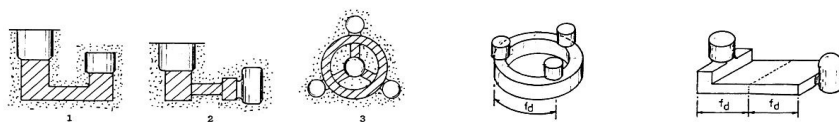
Figure 10. Examples of casting designs requiring separate feeding of sections with different moduli, or to meet feeding distance requirements.
