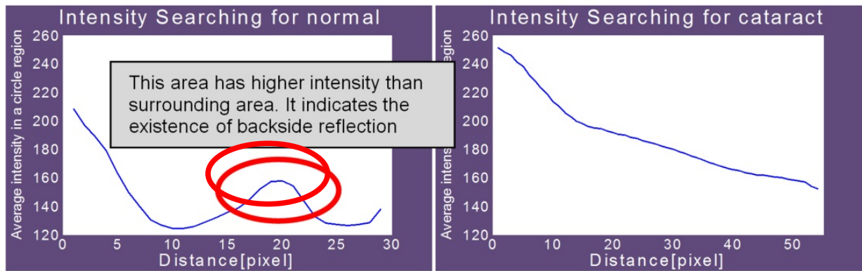
Figure 15. Analyzing backside reflection
