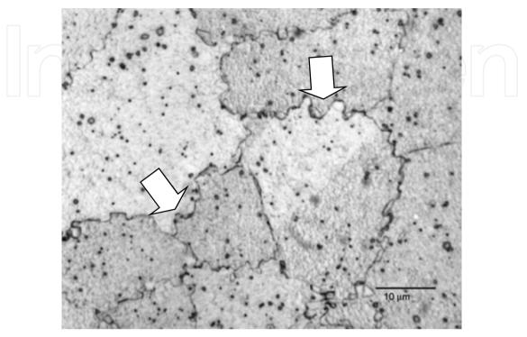
**Figure 16.** Optical microscopy image of serrated grain boundaries. The arrows indicate the serrated boundaries [15]
