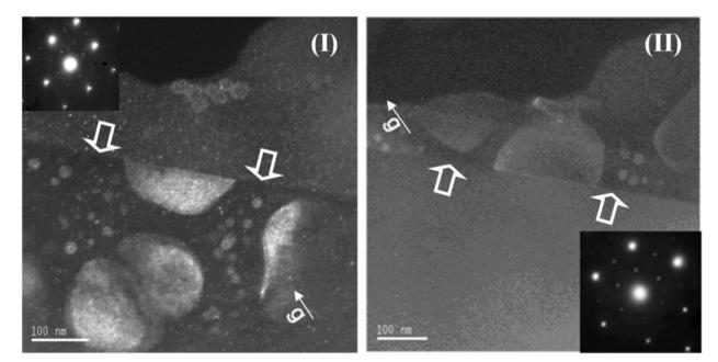
**Figure 18.** A crystallographic analysis of the cutting  $\gamma'$ . The dark field images of the lower and the upper grain are in (I) and (II), respectively. The white arrows indicate the grain boundary
