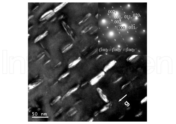
**Figure 5.** TEM DF image of the  $\gamma''$  in IN718. The growth direction is c axis parallel to the a axis of  $\gamma$  ( $(g_{\gamma''} = 0 \ 0 \ 2) \ B = [100]$ ).
