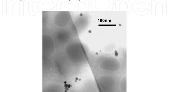
**Figure 17.** General aspect of the high angle grain boundary and  $\gamma'$  (dark spheres). The grain boundary is running diagonally from top left to bottom right
