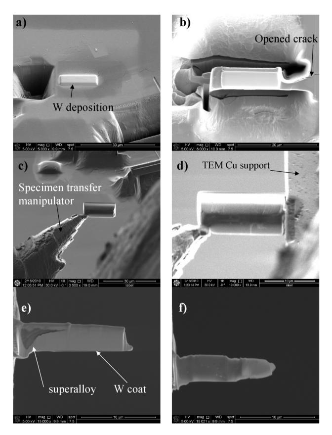
Figure 23. SEM secondary electron images of the process of the site specific TEM sample preparation
