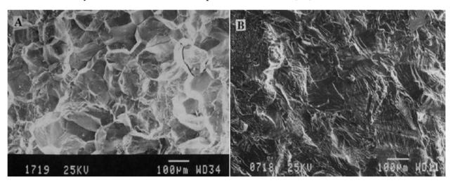
**Figure 15.** Typical intergranular (left) and transgranular (right) fracture surfaces. Alloy 718 tested at 650°C in air (left) and vacuum (right) [18]
