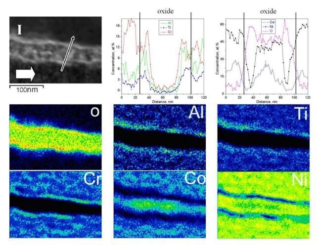
**Figure 25.** STEM dark field image from the region I in Fig. 24 (top left); the thick white arrow indicates the crack growth direction and the thin black arrow indicates the area and the direction of the EDX line scan. The EDX line scan across the oxide (top right) and the EDX mapping results of the oxide (bottom).
