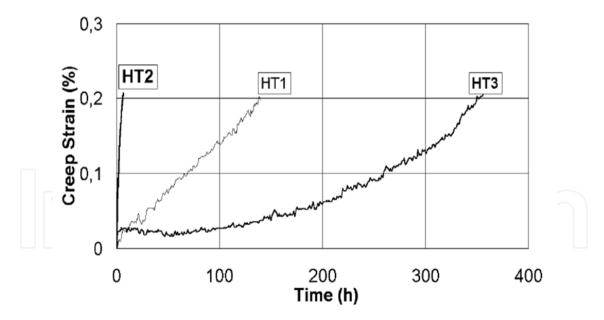
**Figure 14.** Creep strain tested at 700°C for different heat treatments (HT1, HT2 and HT3) The size of  $\gamma'$ : HT2>HT1>HT3 [12].
