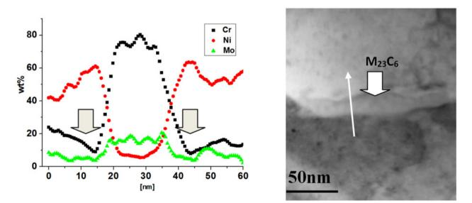
**Figure 9.** Left: STEM EDX line scan results across M<sub>23</sub>C<sub>6</sub> revealed the Cr depletion as indicated by the arrows (Cr nominal composition is 15 wt%). Right: STEM bright field image of the M<sub>23</sub>C<sub>6</sub> (the thin arrow shows the length and the direction of the EDX line scan)
