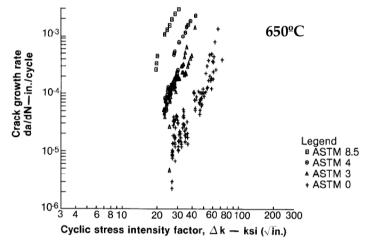
**Figure 12.** UDIMET 720 fatigue crack growth rate for different grain sizes (ASTM grain size between 0 and 8.5: 360µm and 19µm in diameter) tested at 650°C [11]
