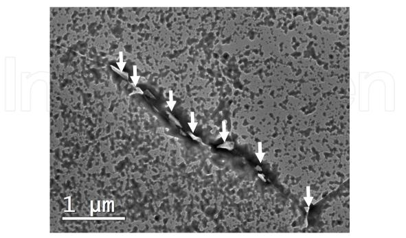
**Figure 7.** Fine M<sub>23</sub>C<sub>6</sub> type carbides precipitate along the grain boundary running diagonally.
