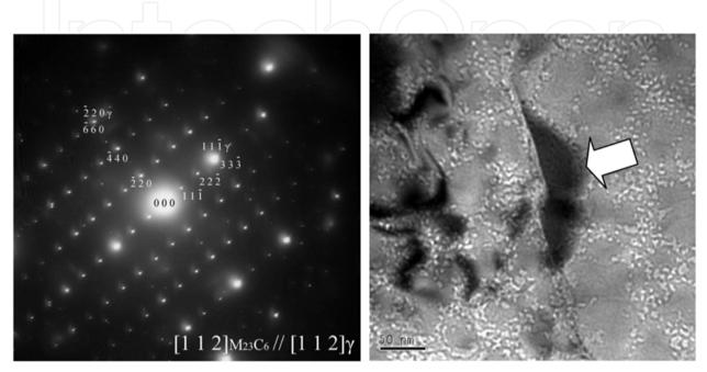
**Figure 8.** M<sub>23</sub>C<sub>6</sub> and  $\gamma$  matrix perfect coherent diffraction pattern (left) and the bright field image from another beam direction to make M<sub>23</sub>C<sub>6</sub> outstanding (right)
