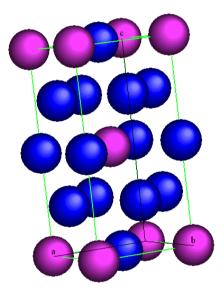
**Figure 3.**  $\gamma$ '' D0<sub>22</sub> structure. Ni atoms are blue and Nb, Al and Ti purple
