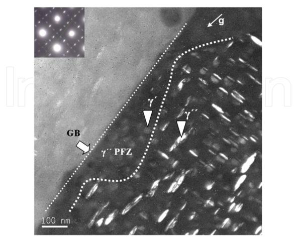
**Figure 20.**  $\gamma''$  PFZ appeared in IN718, although  $\gamma'$  still exist in the  $\gamma''$  PFZ adjacent to the grain boundary
