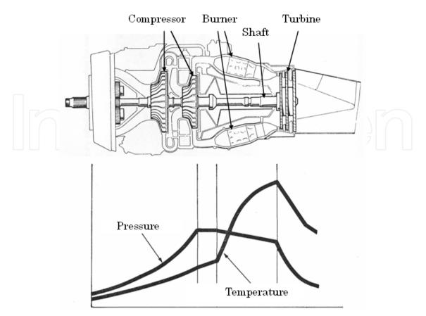
**Figure 1.** (a) Schematic diagram of a turbine engine Ref. [3]. (b) Schematic diagram of the temperature and pressure gradients throughout the engine component correlating with the diagram (a) Ref. [4]
