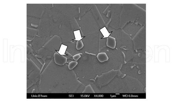
Figure 6. Coarse Nb and Ti based carbide in IN718
