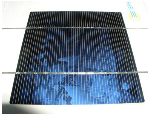
Figure 4. With In-Laminate Laser Soldering (ILLS) manufactured solar cell module. Adapted from [35].
