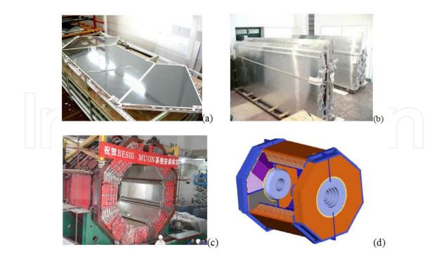
**Figure 8.** a). The RPC moduls, (b). The Suprlayer Modul, (c). The overview the barrel part of the MUC detector after it's assemblage, (d) The construct of the BESIII MUC detector.
