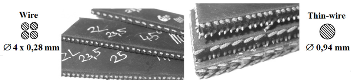
Figure 20. Single-layer specimens of steel-cord belt with wire cord and two-layer specimens with thin-wire cord (right)
