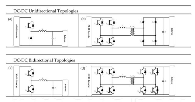
**Figure 5.** Main DC-DC power converters topologies used in EVs batteries charging systems: (a) unidirectional buck converter; (b) unidirectional isolated converter; (c) bidirectional buck boost converter; (d) bidirectional isolated converter.
