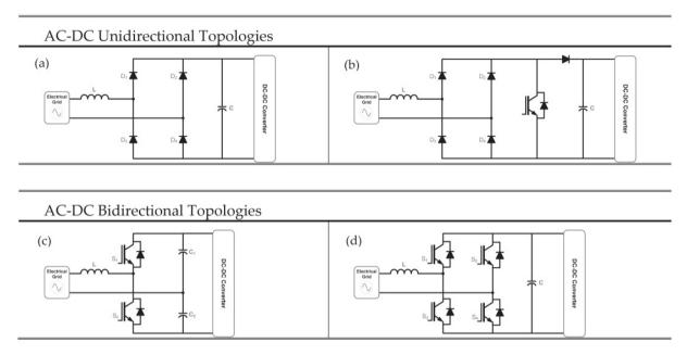
**Figure 4.** Main AC-DC power converters topologies used in EVs batteries charging systems: (a) unidirectional full-bridge non-controlled converter; (b) unidirectional full-bridge non-controlled converter followed by a boost converter; (c) bidirectional half-bridge full-controlled converter; (d) bidirectional full-bridge full-controlled converter.
