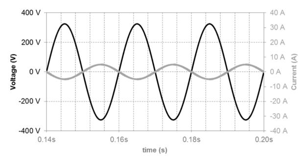
Figure 11. Typical current waveform of an AC-DC power electronic converter with sinusoidal current, delivering energy back to the power grid.
