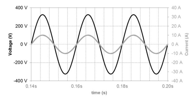
Figure 9. Typical current waveform of an AC-DC power converter with sinusoidal current consumption.
