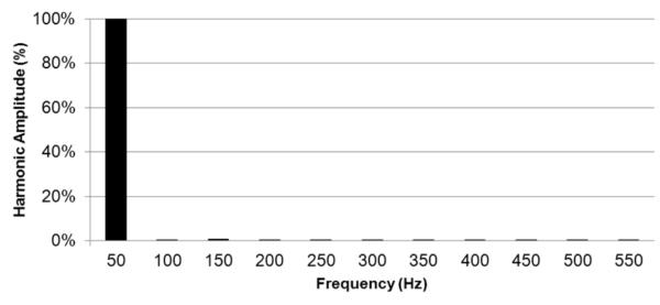
Figure 12. Harmonic spectrum of the typical current waveform of an AC-DC power converter with sinusoidal current, delivering energy back to the power grid.
