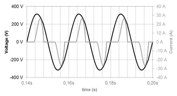
**Figure 7.** Typical waveforms of a conventional AC-DC power converter.
