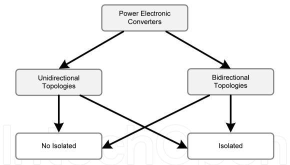
Figure 3. Main categories of AC-DC power converters topologies used in EVs batteries charging systems.
