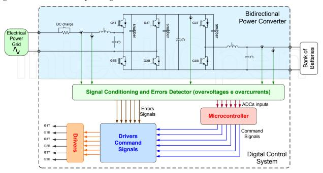
Figure 13. Schematic of the developed Electric Vehicle batteries charging system.
