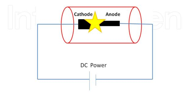
Figure 3. Schematic diagram of apparatus for preparing CNTs.
