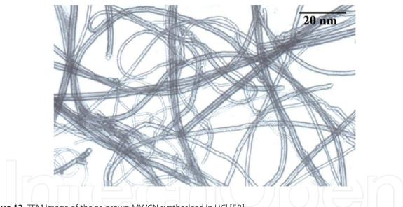
Figure 12. TEM image of the as-grown MWCN synthesized in LiCI [58].
