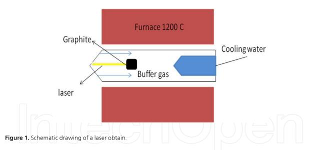
The target is vaporized in high-temperature buffer gas like Ar and formed CNTs. The produced CNTs are conveyed by the buffer gas to the trap, where they are collected. Then CNTs can be found in the soot at cold end.
