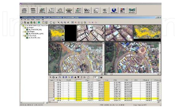
Fig. 4. Selecting the control points for rubber-sheeting method for image geo-referencing (AutoSync module of ERDAS Imagine).
