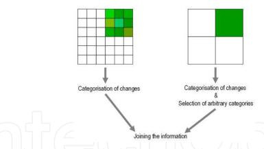
Fig. 8. Change detection approach takes into account the neighbourhood and change information by joining different spatial scales.
