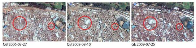
Fig. 3. Examples of rooftops, rooftops renovations and buildings constructions on VHR satellite imagery from three different dates.
