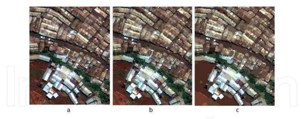
Fig. 6. Original GeoEye image (a), objects segmented (b), objects merged (c) (Feature Extraction module of ENVI EX).
