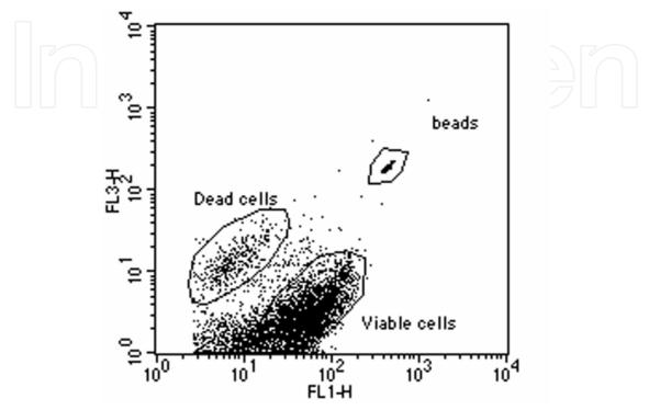
Fig. 8. Dot plot FL1 vs. FL3 of a marine sample stained with SYBR Green I and PI
