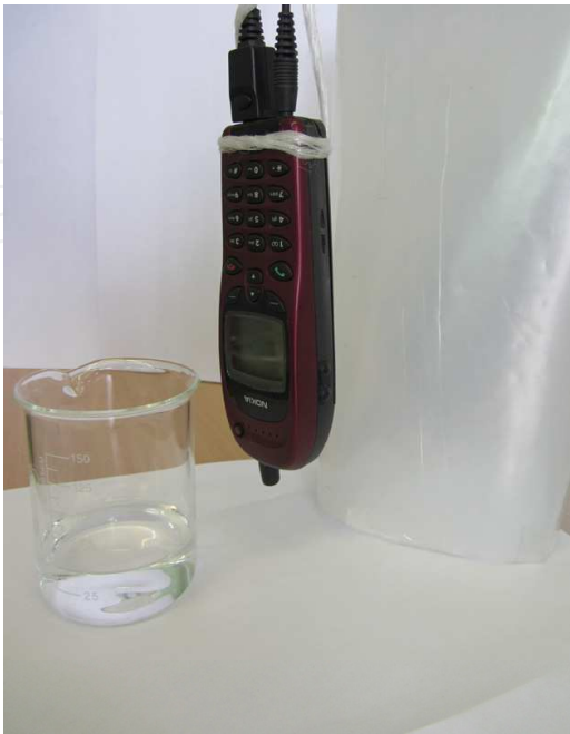
Fig. 7. The process of exposing two water samples to the MP radiation. One of the glasses is wrapped by thin (40μm) four-layered PF. The exposure duration is 1.5 hour.
