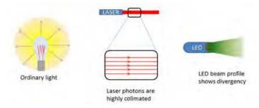
Fig. 5. Illustration shows emitted beam propertes of ordinary light, laser and LED light
