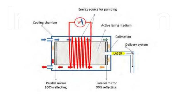
Fig. 2. Laser system illustration
