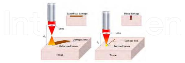
Fig. 16. Focusing and defocusing. Laser beam creates deeper impact at a narrow diameter at surface when focused. If defocused, damage depth is more superficial but damage area on the surface is wider. To defocus the beam  $d_1 < d_2$ .
