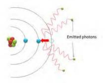
Fig. 3c. Photons are emitted while excited atom are returning to ground state following excitation phase.
