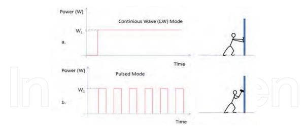
Fig. 8. Working modes of laser. Line graphic show (a.) continuos wave and (b.) pulsed beam profiles.
