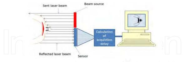
Fig. 11. Laser scanning process. Laser beam is sent to the surface to be scanned and distance between source and arget is calculated with reflection time. Computed raw data helps to reconstruct target surface topography 3 dimentionally.
