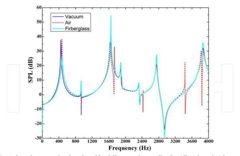
Fig. 6. Sound pressure levels radiated by different orthogonally rib-stiffened sandwich structures plotted as functions of frequency for stiffener separations ( $l_x$ ,  $l_y$ ) = (0.20m, 0.20m)
