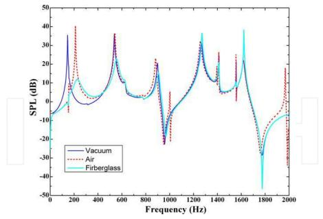
Fig. 7. Sound pressure levels radiated by different orthogonally rib-stiffened sandwich structures plotted as functions of frequency for stiffener separations ( $l_x$  =0.35m,  $l_y$  =0.35m)
