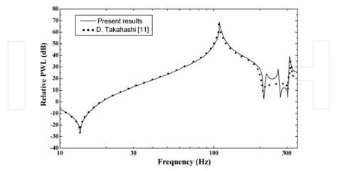
Fig. 5. Comparison between model predictions and theoretical results of Takahashi [11] for ribstiffened double-panel structure excited by time-harmonic point force at location  $(l_x/2, l_y/2)$
