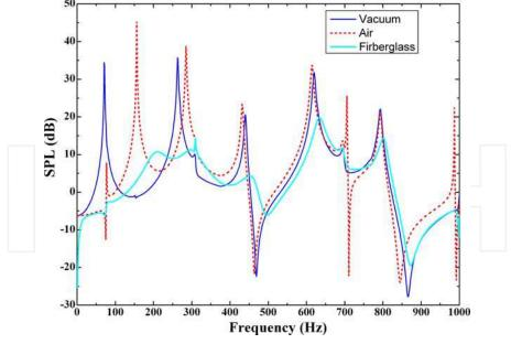
Fig. 8. Sound pressure levels radiated by different orthogonally rib-stiffened sandwich structures plotted as functions of frequency for stiffener separations ( $l_x$  =0.50m,  $l_y$  =0.50m)
