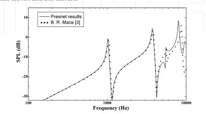
Fig. 4. Comparison between present model predictions and those by Mace [3] for orthogonally rib-stiffened single panel excited by time-harmonic point force at location (0, 0)
