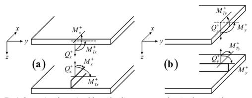
Fig. 2. Conventions for tensional forces, bending moments and torsional moments between upper panel and (a) x-wise and (b) y-wise stiffeners, which also hold at the interface between bottom panel and x- and y-wise stiffeners
