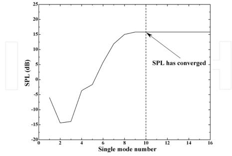
Fig. 3. Convergence check of numerical solution for sound radiation of an infinite orthogonally rib-stiffened sandwich structure with stiffener separations ( $l_x$ ,  $l_y$ ) = (0.20m, 0.20m) when excited by a harmonic point force at 10 kHz
