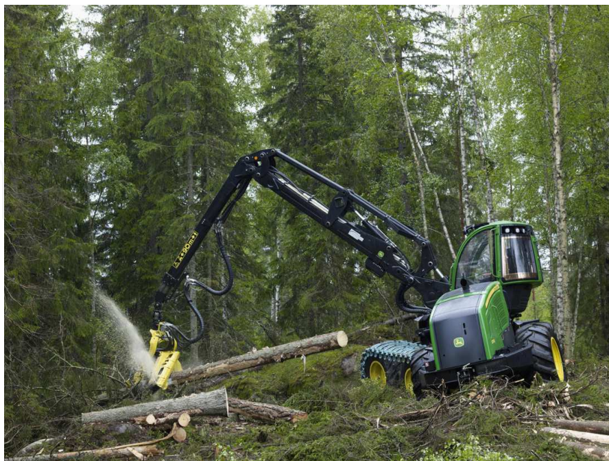
Fig. 1. Harvester John Deere 1270E with a rotating cab
