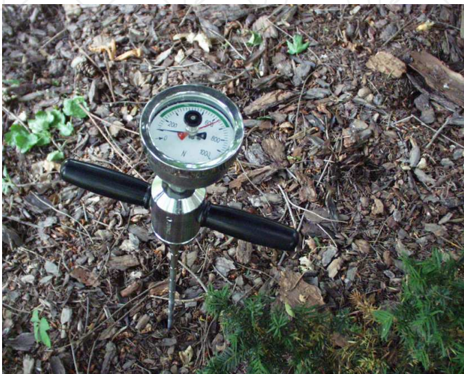
Fig. 7. Measurement of soil resistance by penetrometer
