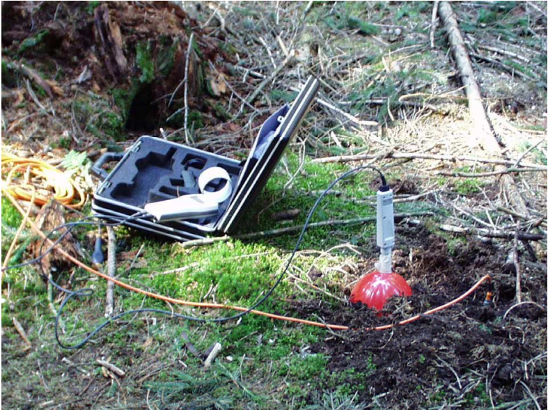
Fig. 4. Upper panel - Concentration of CO 2 in soil air in a crossing line after several harvester passages (soil moisture: 35%). Lower panel – CO 2 measurement in control line with GMP 221 Carbon dioxide probe (Vaisala, Finland)
