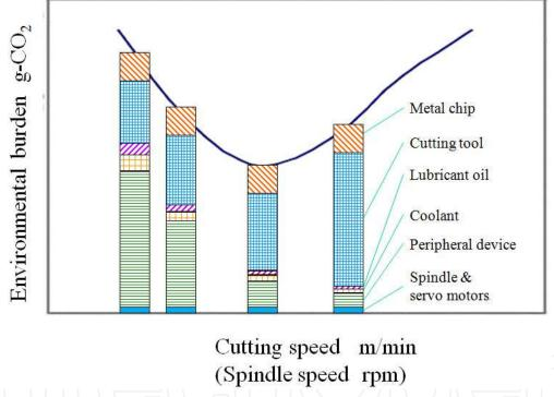
Fig. 6. Tendency due to high speed milling
