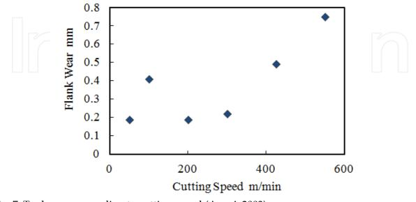
Fig. 7. Tool wears according to cutting speed (Anzai, 2003)
