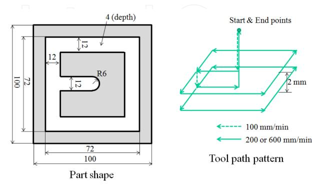
Fig. 4. Part shape and tool path pattern
