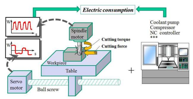
Fig. 2. Electric consumption model for machine tool
