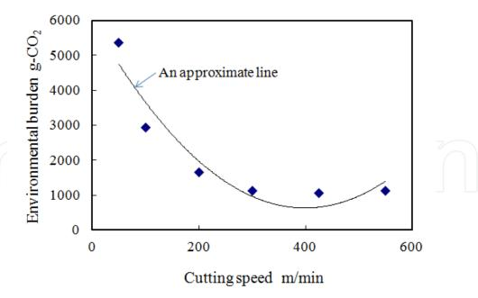
Fig. 8. Environmental burden vs. cutting speed
