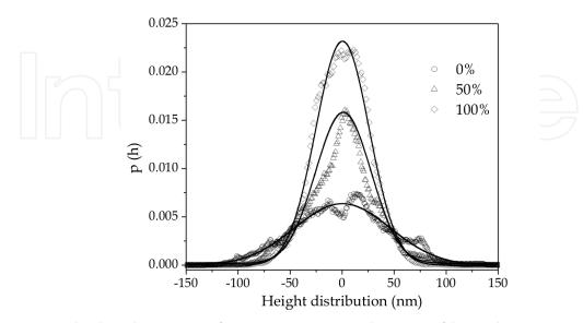
Fig. 9. Height distribution p(h) for ST0%, ST50% and ST100% films. The continuous line represents adjustments, using the Gaussian function (Eq. 4).
