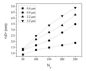
Fig. 5. Average distance  $\langle d \rangle$  (Eq. 9) in function of the first-neighbor selected peaks, 50, 100, 1500, 200, and 250, for sample thickness of 0.4, 0.9, 2.2, and 3.2 µm.
