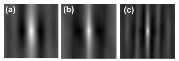
Fig. 10. Height auto-covariance image of casting PVDF/PPV films stretched at (a) 0%, (b) 50%, and (c) 100% for the AFM images in Fig. 8.
