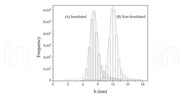
Fig. 17. Histogram of peak heights in irradiated (a) and non-irradiated (b) regions. Gaussian function was used to fit the distribution.
