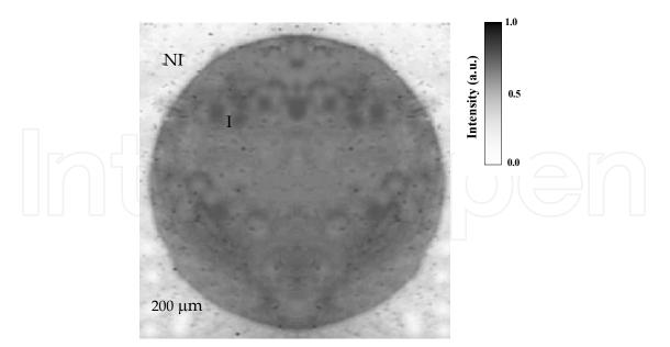
Fig. 14. Optic image of non-irradiate (NI) and irradiate (I) region.
