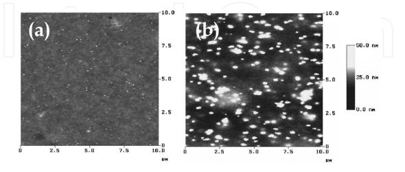
Fig. 2. AFM height image for *casting* PPV films with different thickness: (a)  $0.4\mu$ m and (b)  $3.2\mu$ m.
