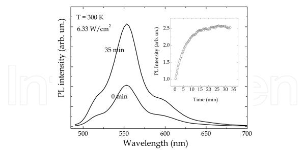
Fig. 15. PL spectra before (0 min) and after (35 min) photo-irradiation at 200 mW/cm<sup>2</sup> for a PPV cast film under environmental conditions. The insert shows the time evolution of the PL-intensity.
