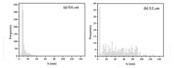
Fig. 3. Height histogram of AFM images in Figure 2, with thickness of (a)  $0.4\mu m$  and (b)  $3.2 \mu m$ .
