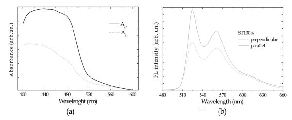
Fig. 12. (a) Polarized absorbance spectra for casting PVDF/PPV film stretchered at 100% (ST100%) parallel (A<sub>//</sub> - black line) and perpendicular (A<sub>⊥</sub> - red line) to the stretching direction. (b) Polarized photoluminescence spectra for casting PVDF/PPV film stretched at 100% (ST100%) parallel (black line) and perpendicular (red line) to the stretching direction.
