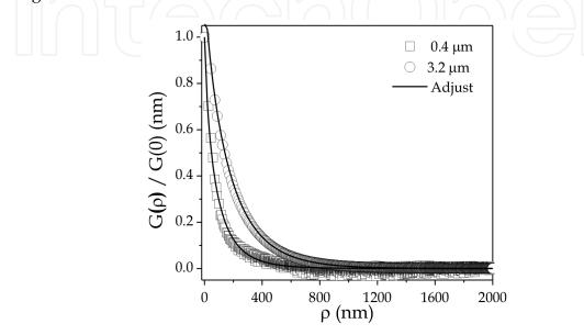
Fig. 6. Height auto-covariance curves for the AFM image (Fig. 1) for casting PPV films thickness of 0.4  $\mu$ m (open cube) and 3.2  $\mu$ m (open circle). The continuous line represents the adjustment using a self-affine equitation (Eq. 10c).
