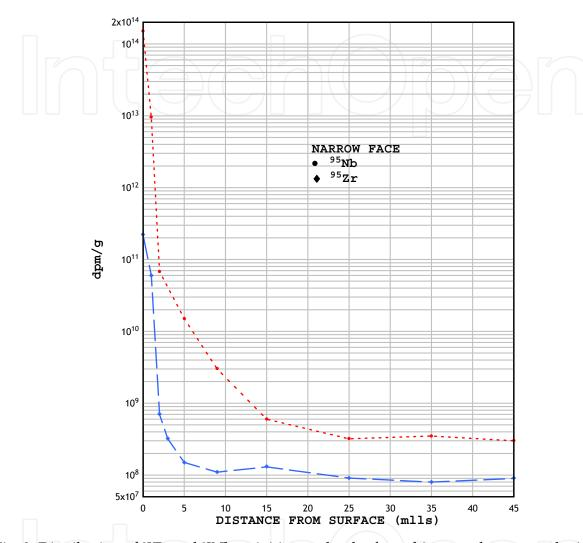
Fig. 3. Distribution of 95Zr and 95Nb activities on depth of graphite sample contacted with salt melt in the reactor MSRE core (Kirslis & Blankenship, 1969)
