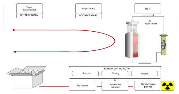
Fig. 4. Scheme of fragment 99Mo production in a molten salt reactor
