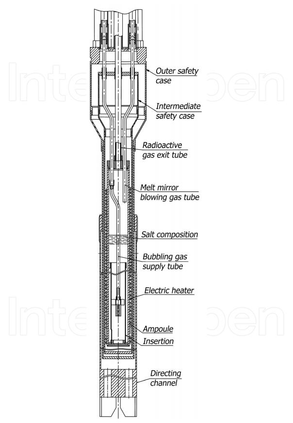
Fig. 5. General scheme of the ampoule part of the loop system "RAMUS"
