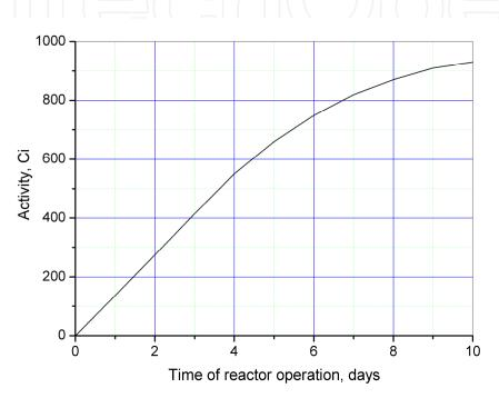
Fig. 6. Activity of 99Mo in the core depending on reactor operating time
