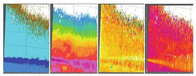
Fig. 5. RHI scans north of Vantaa radar 30 August 2009 00:45 UTC. . Range 100 km, height 10 km, parameters from left to right: Hydrometeor classification, reflectivity Z, differential reflectivity ZDR and copolar correlation factor RhoHV.
