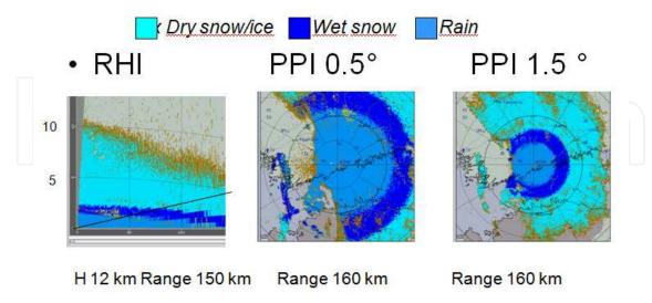
Fig. 1. Hydrometeor classification 30 August 2009 00:45 UTC in Vantaa, Finland. RHI to 150 km in range, 12 km in height (left). PPI to 160 km in range, 0.5 degrees in elevation (middle) and 1.5 degrees in elevation (right). Cyan for dry snow, dark blue for melting snow, light blue for rain.
