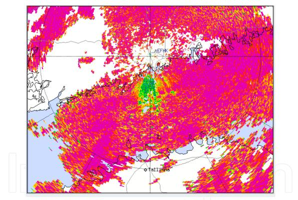
Fig. 4. Sea clutter and lake effect snow seen with polarimetric parameter RhoHV. RhoHV over 0.98 in snow, less than 0.8 in sea clutter. The range ring indicates 100 km from the radar.
