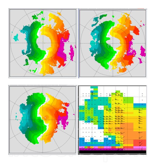
Fig. 8. PPI images of Doppler velocity 30 minutes apart (5:00, 5:30 and 6:00) and time series of wind and reflectivity profiles 02:00 to 07.00 UTC 14 January 2008. Green colours towards radar, reds and yellows away. Reflectivity from -20 dBZ (blue) to +20 dBZ(purple)
