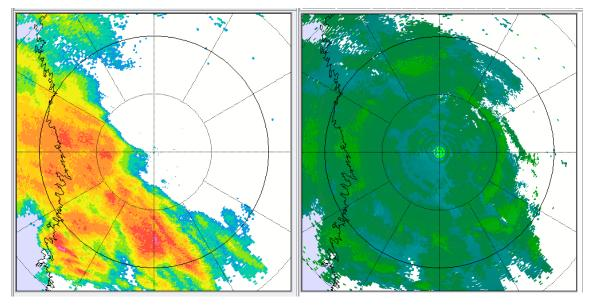
Fig. 7. CAPPI at 500 m height on left, TOPS with threshold -10 dBZ on right. 14 January 2008 05:30 UTC, precipitation on the surface had not yet reached the radar location. Range rings at 50 and 100 km from radar, reflectivity scale as in Fig. 2., green shades for tops in steps of 2 km.
