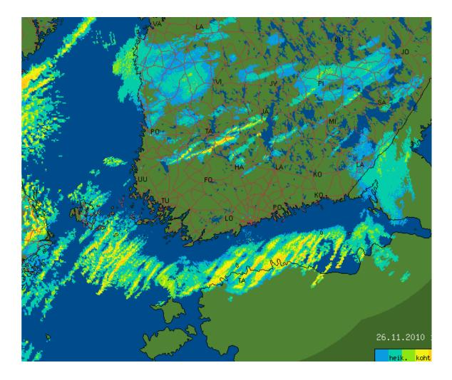
Fig. 10. Lake effect snow 26.11. 2010 10 UTC. Pseudo-CAPPI reflectivity composite of 5 Finnish and 2 Swedish radars at nominal height of 500 m.
