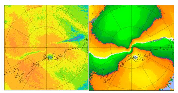
Fig. 3. A Doppler snake case 17 March 2005 03:00 UTC. PPIs of reflectivity (left) and Doppler velocity (right). Wind is from south-southeast, warm colours indicate echoes moving away from the radar and cold colours towards the radar . The velocity field is folded, unambiguous speed 7.6~m/s. A band of weaker reflectivities cutting through the image from southwest to east, at same location as zero Doppler speeds (white). Reflectivity colour scale as in Fig. 2.
