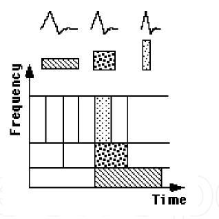
Fig. 2. Wavelet time-frequency plane ((Graps, 1995) with minor modifications)
