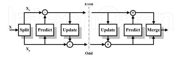
Fig. 16. Lifting-based Wavelet Transform
