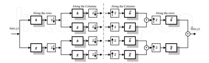
Fig. 12. Two-dimensional Mallat's analysis and synthesis tree
