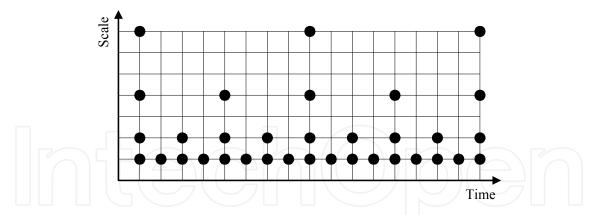
Fig. 5. Dyadic wavelet transform space representation
