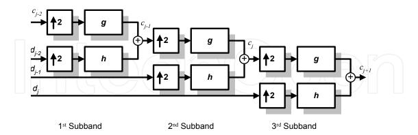
Fig. 9. Three-Stage synthesis Subband Coding
