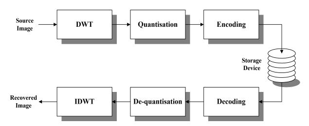
Fig. 21. Wavelet-based encoding scheme
