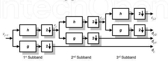
Fig. 7. Three-Stage analysis Subband Coding
