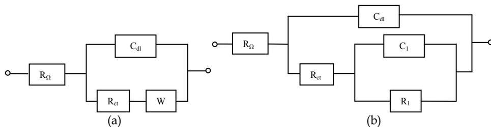
Fig. 8. Equivalent circuit of EIS for different samples.
