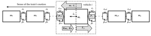
Fig. 14. Mechanical model of the train
