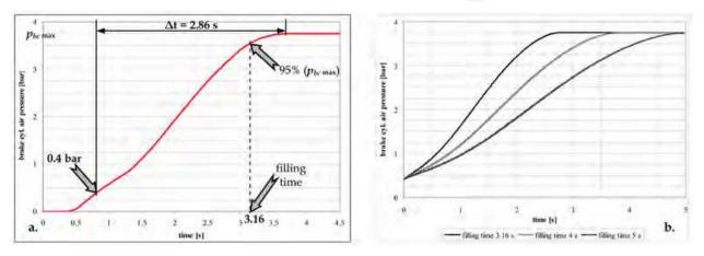
Fig. 19. Air distributor filling characteristics: a – experimentally determined; b – extrapolated functions.
