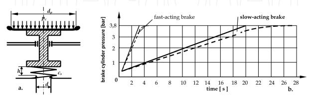
Fig. 18. Influence of valve opening on filling characteristics: a – schematic of pressure-spring controlled valve; b – theoretical filling characteristics (dotted line: valve controlled filling).
