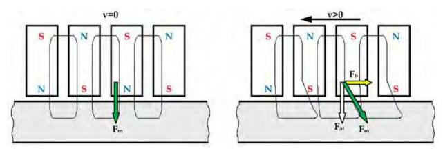
Fig. 8. Principle of eddy current brake system ( $F_m$  – magnetic force;  $F_{at}$  – attraction force;  $F_b$  – braking force).
