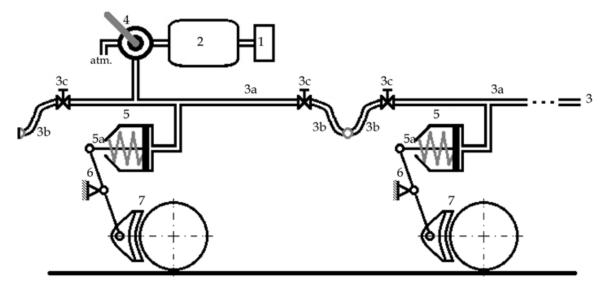
Fig. 1. Schematic of straight compressed air brake system: 1 – compressor; 2 – main reservoir; 3 – train's brake pipe; 3a – vehicle's brake pipe; 3b – flexible coupled hoses; 3c – angle cock; 4 – driver's brake valve; 5 – brake cylinder; 5a – piston rod; 6 – brake rigging; 7 – brake shoe.
