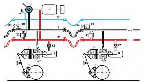
Fig. 4. Schematic of electro-pneumatic brake system: 1 – compressor; 2 – main reservoir;
