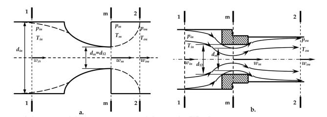
Fig. 17. Model of nozzle: a - ideal convergent nozzle; b - real circular calibrated orifice.
