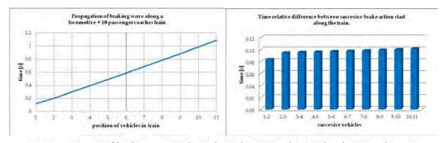
Fig. 16. Propagation of braking wave along the a short train (particular theoretical case study).
