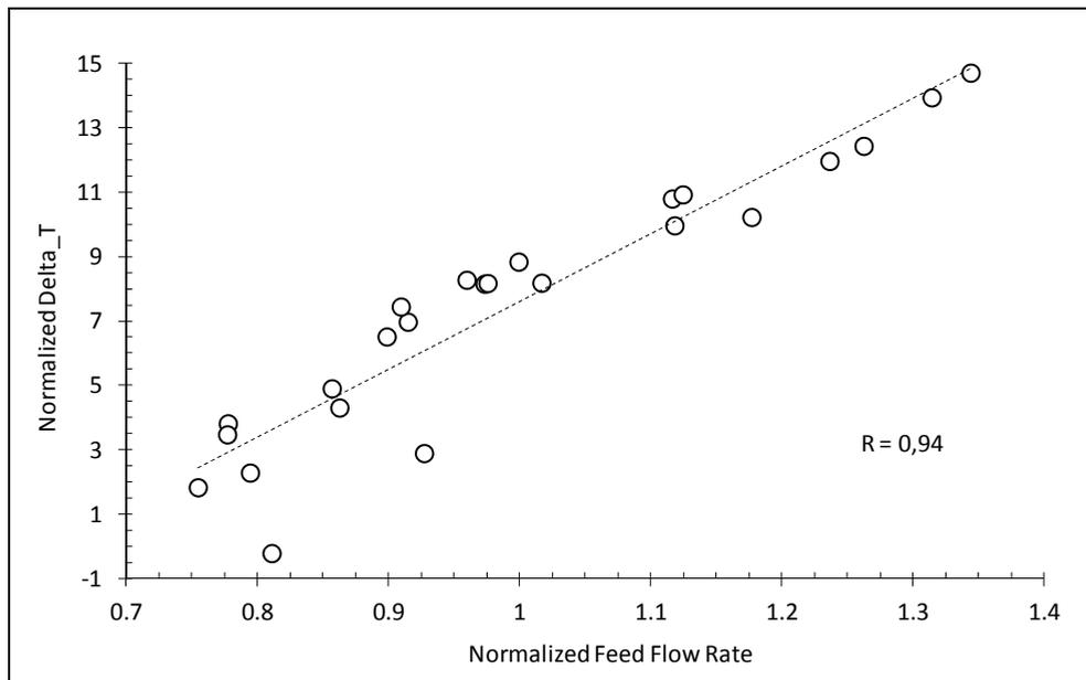
Fig. 5.3. Historical data: Delta\_T versus feed flow rate.
