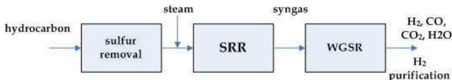
Fig. 1.1.1. Hydrogen generation unit – process block diagram.
