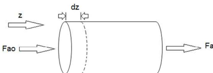
Fig. 2.2.1. Reactor differential volume representation.
