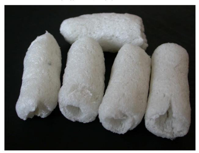
Fig. 1. Extruded starch foams.
