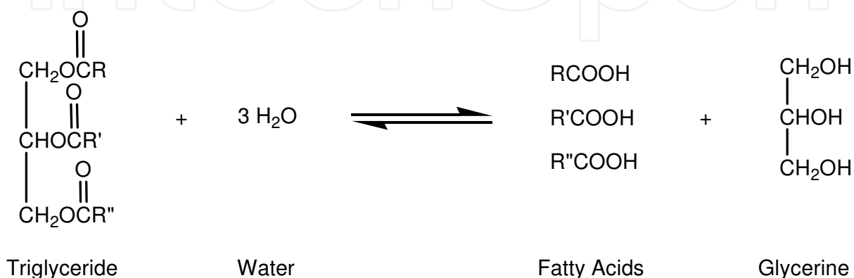
Fig. 1. Splitting or hydrolysis of fat or oil triglycerides to fatty acids and glycerine
