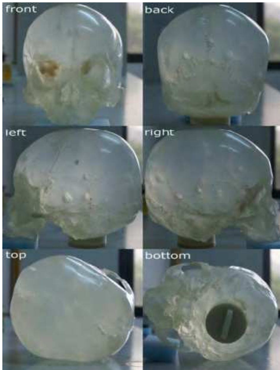
Fig. 5. The visualization skull model by the PC resin on the molds technology [8]
