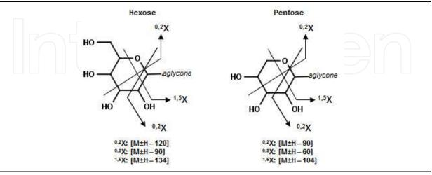
Table 2. Characteristic mass losses of flavonoid glycosides and characteristic cross-ring cleavages in the sugar rings of hexoses and pentoses (Vukic & Guttman, 2010; Cuyckens & Claeys, 2004).
