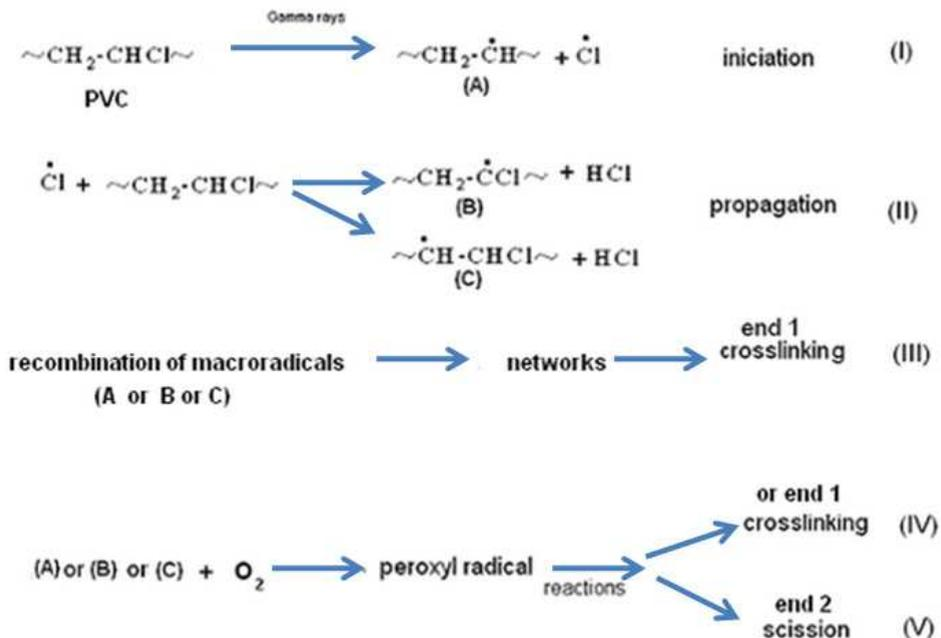
Fig. 7. Effects of gamma irradiation on PVC molecule
