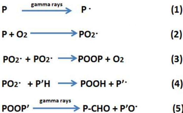
Fig. 10. Polyolefins oxidation caused by gamma sterilization
