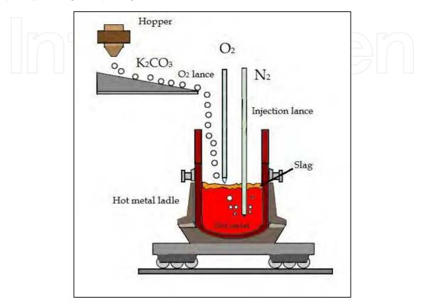
Fig. 4. Production of potassium silicate fertilizer from steelmaking slag (Takahashi, 2002).
