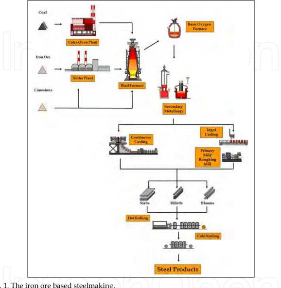
Fig. 1. The iron ore based steelmaking.
