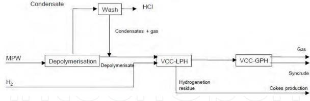
Fig. 11. Veba Combi Cracking process (Sas, 1994).
