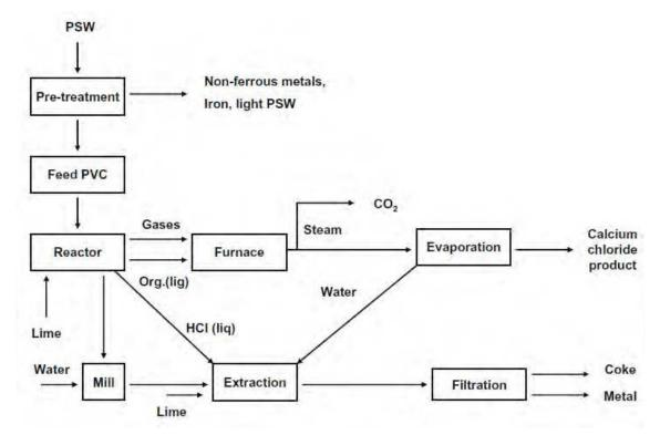
Fig. 8. NTK process diagram (Tukker et al., 1999).
