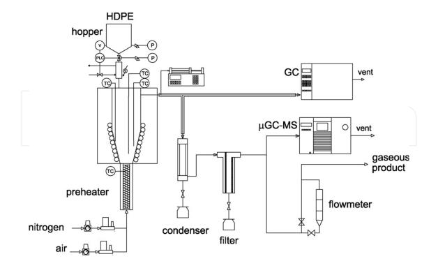
Fig. 3. Schematic representation of the continuous pyrolysis unit (Elordi et al. 2009).
