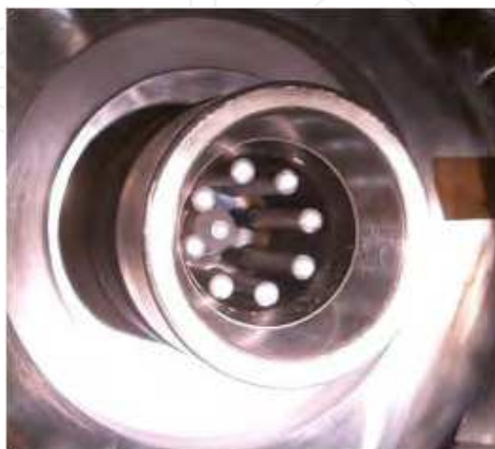
Fig. 8. Magnetoplasmadynamic(MPD) arcjet as solar wind simulator (SWS).
