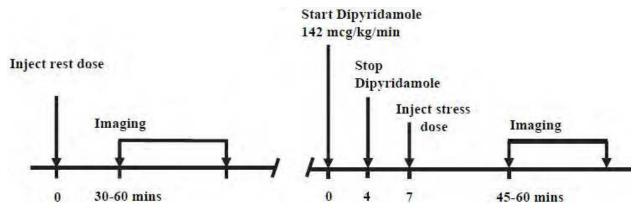
Fig. 8. Tc-99m imaging protocols: One-day rest/dipyridamole pharmacologic stress.
