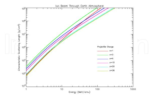
Fig. 16. Characteristic scattering length for ion beam transport through the Earth's atmosphere. The charge number (z) of the ion is specified in the legend.
