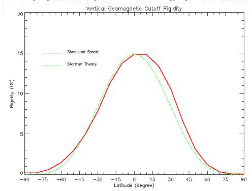
Fig. 10. Zonal-averaged vertical geomagnetic cutoff rigidity. The solid red line corresponds to the quiescent cutoff rigidities computed from particle trajectories and the IGRF model. The green dotted line is the analytical solution for the vertical cutoff rigidity using Störmer Theory.
