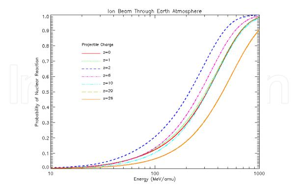
Fig. 19. Nuclear survival probability versus kinetic energy of an ion beam incident at the top of Earth's atmosphere. The charge number (z) of the ion is specified in the legend.
