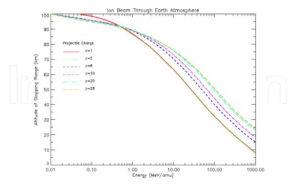
Fig. 18. Average range versus kinetic energy of an ion beam incident at the top of Earth's atmosphere. The charge number (z) of the ion is specified in the legend.
