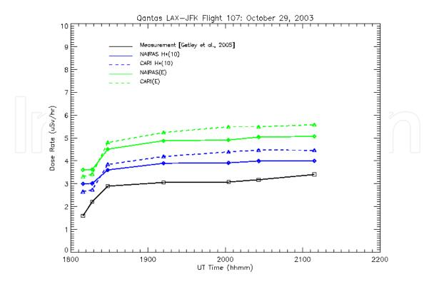
Fig. 25. Comparisons between NAIRAS, FAA/CARI, and TEPC measurements for Qantas Flight 107 from Los Angeles, California to New York, New York on October 29, 2003. The dosimetric quantities compared are effective dose rate (denoted E) and ambient dose equivalent rate (denoted H\*(10)).
