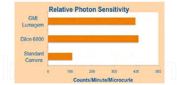
Graph 1. The relative photon sensitivity of commercially available, breast-optimized imaging systems compared to that of the standard gamma camera.
