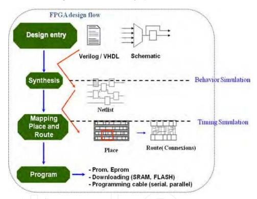
Fig. 14. *FPGA* design flow overview.
