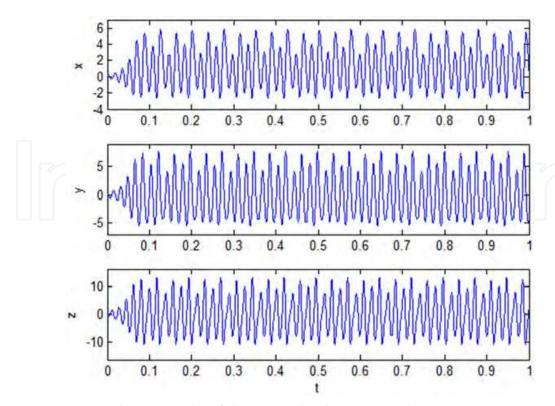
Fig. 7. *MatLab* simulation results of the *x*, *y* and *z* chaotic signals.
