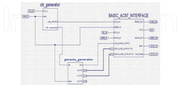
Fig. 20. Functional blocks implemented in the *FPGA* chip.
