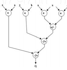
Fig. 16. *RTL* architecture of the *Q* functional units.
