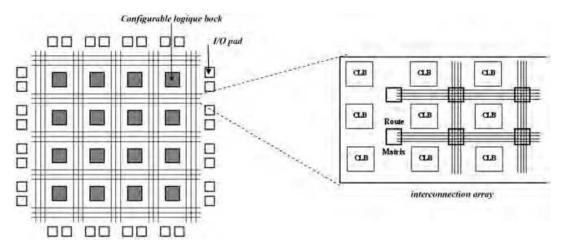
Fig. 9. Overview of the inner architecture of a FPGA.
