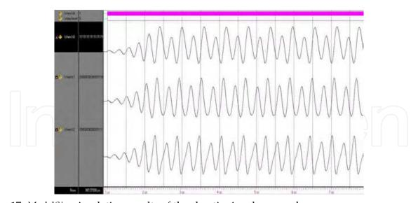
Fig. 17. ModelSim simulation results of the chaotic signals x, y and z.
