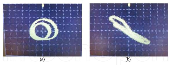
Fig. 22. Real-time measurement results of (a) the (x-y) chaotic attractor, and (b) the (x-z) chaotic attractor.
