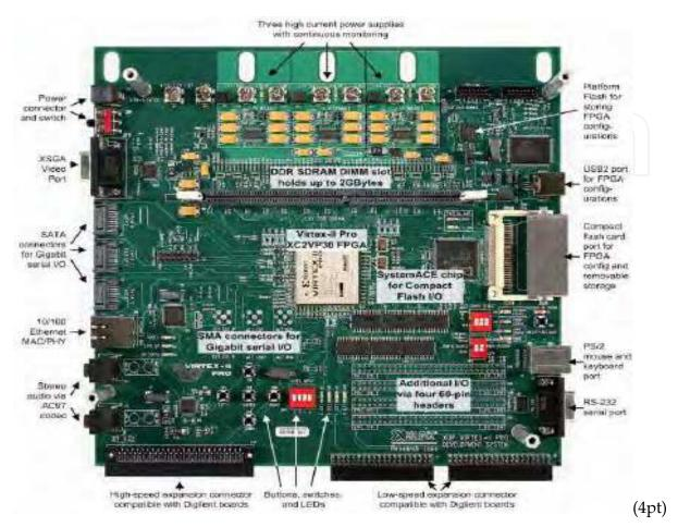
Fig. 18. XUP Xilinx Virtex-II Pro embedded platform.
