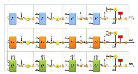
Fig. 15. RTL architecture of the Genesio-Tesi chaotic system.
