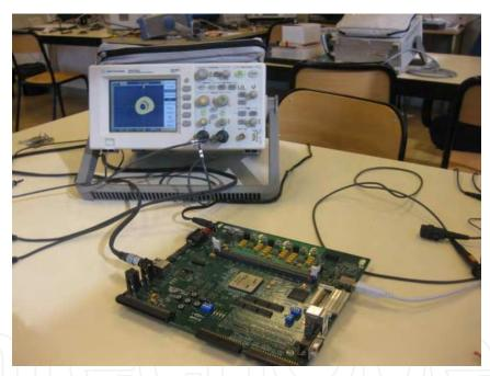
Fig. 23. Photo of the experimental hardware implementation and measurements of the *Genesio-Tesi x-y* chaotic attractor.
