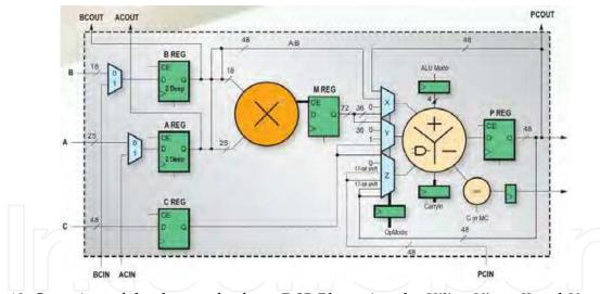
Fig. 13. Overview of the data-path of one *DSP*-Bloc using the *Xilinx Virtex II* and *V* technologies [Xilinx2, 2007; Xilinx3, 2000; Xilinx, 2008].
