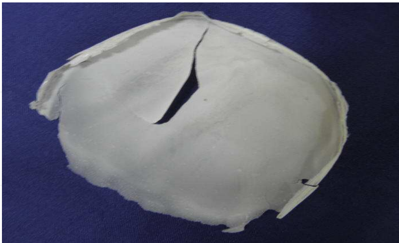
Fig. 9. Biopolymer of PHB obtained from Bacillus aryabhatai
