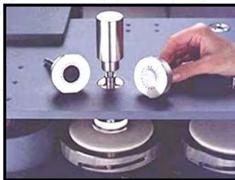
Fig. 16. Setting of sock kit on Martindale apparatus
