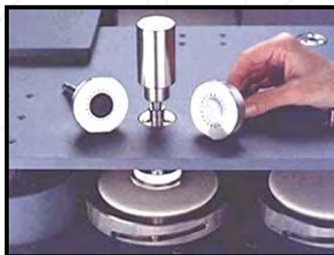
Fig. 16. Setting of sock kit on Martindale apparatus
