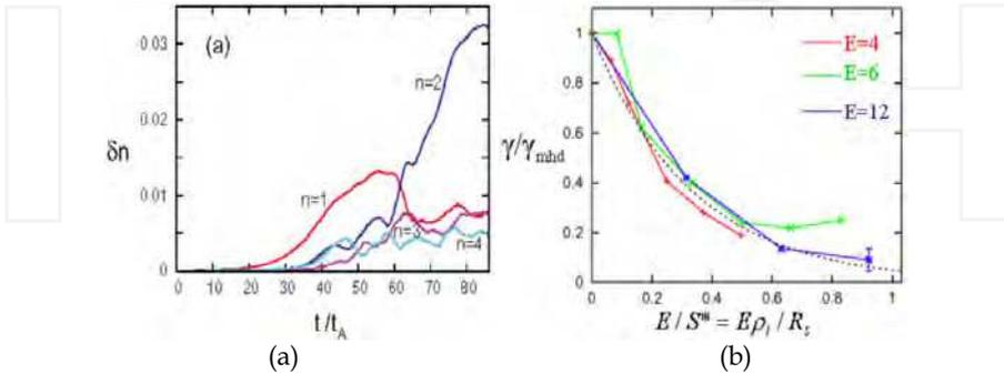
Fig. 9. (a) Time evolution of the amplitudes of different  $n$ -modes in prolate FRC with  $S^* = 20$  and (b) Growth rate of  $n = 1$  tilt instability for three elliptical FRC equilibria with  $E = 4, 6$  and  $12$
