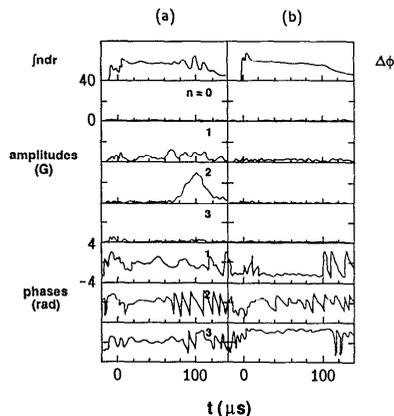
Fig. 7. Toroidal Fourier analysis of the  $B_\theta$  for good confinement. The Fourier amplitudes and phases are shown as functions of time for (a) even and (b) odd components. The top trace of (a) is a line-integrated electron density and (b) diamagnetism.
