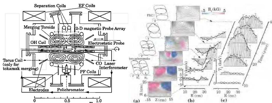
Fig. 4. (a) TS-3 merging device and 2D contours of poloidal flux surface and toroidal magnetic field on the R-Z plane; radial profiles of (b) ion toroidal velocity  $V$ , and (c) ion temperature ( $T_i$ ), on the midplane, during the counter helicity merging of two spheromaks with equal but opposing  $B_t$ . The red and blue colors indicate the positive and negative amplitudes of  $B_t$ .
