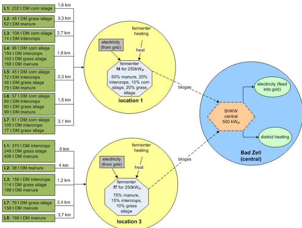
Fig. 5. PNS optimum structure with a central 500 kW<sub>el</sub> CHP
