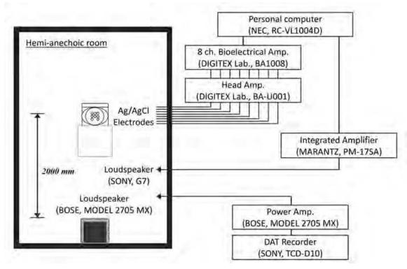
Fig. 2. Block diagram of experimental system
