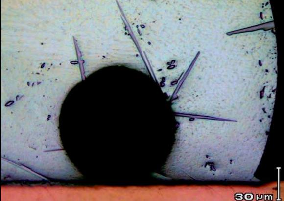
Fig. 4. As-solidified microstructure of a Sn3.0Ag0.5Cu solder interconnection illustrate how the primary  $Cu_6Sn_5$  particles have nucleated on oxide particles on the surface of the liquid.
