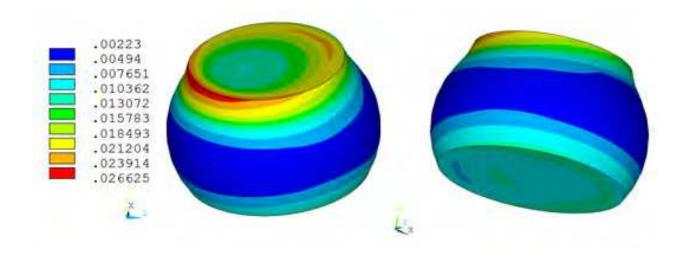
Fig. 5. Calculated strain energy density of the cornermost solder interconnections of the component board assembly sketched in Figure 1 [63,64].
