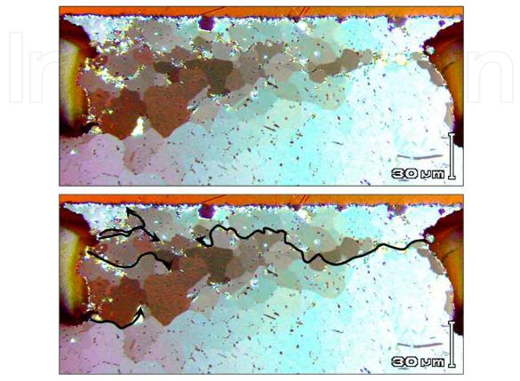
Fig. 10. Cracks propagate intergranularly between the recrystallized grains: a) cross-section of a recrystallized and cracked solder interconnection; b) the same image as in (a) but with superimposed crack paths.
